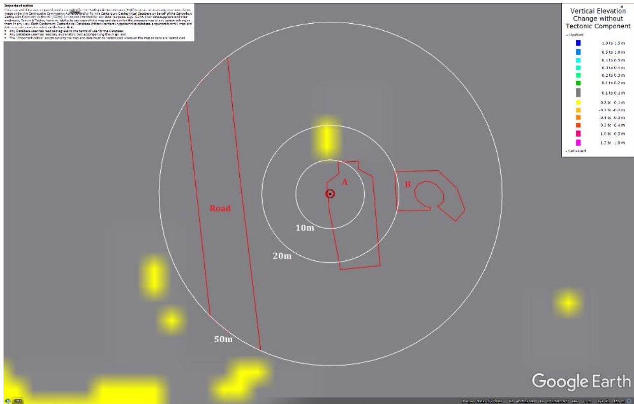
Figure 28: Ground surface subsidence without tectonic component for June 2011 Earthquake according to the LiDAR DEM.
